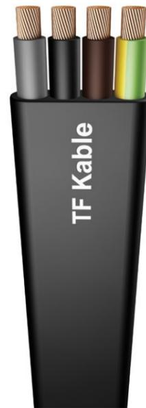
**Applications:** Flexible flat cable designed for mechanical stresses, especially for applications with frequent bending during operation and for bending in one plane only. The cable is used on festoon systems and for connecting moveable parts of machine tools, material handling equipment. Usable in wet or dry conditions, outdoors and indoors.
