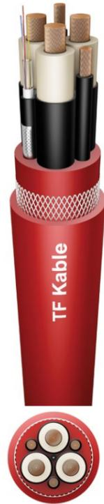
**Applications:** Specially designed flexible reeling cable with reduced dimensions for extremely high mechanical stresses occur in applications with mono spiral reels and cylindrical reels, very high reeling speed, torsional stress. Also for connection of large material handling machines such as excavators, dumpers, crushers in opencast mines. Usable in wet or dry conditions, in industrial units, in underground and opencast mining, in explosion-risk areas.
