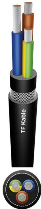
**Applications:** Flexible cable designed for high mechanical stresses, especially for applications with frequent winding and unwinding with co-occurrent tensile and torsion stress. The cable is used for conveyors, container cranes, harbour cranes, building machinery, handling machines in mining and tunnelling equipment. For use in wet or dry conditions, in industrial units, in underground and open-cast mining, in explosion-risk areas.
