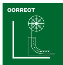
The cable should be fed at the center point above the cable guide, regardless of one or two-way guidance.
