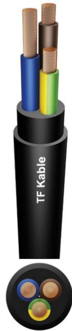
**Applications:** Flexible cable designed for high mechanical stresses, especially for applications with frequent bending. For festoon systems and connecting moveable parts of container cranes, industrial units, material handling equipment. For use in wet or dry conditions, outdoors, indoors.
